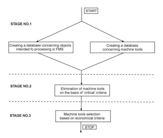
Fig. 3. Diagram of the selection FMS machine tools subsystem
