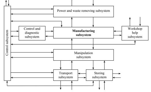
Fig. 1. Functional FMS subsystems [5]
